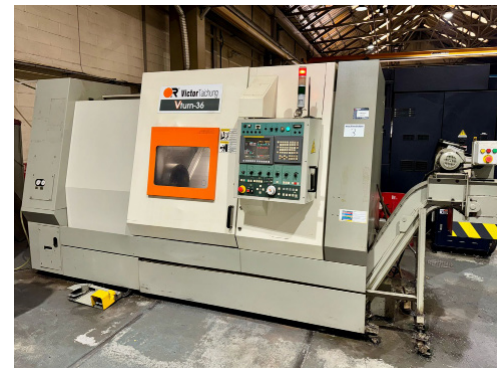
Lot 3: VICTOR VTURN 36/85 CNC Lathe with Fanuc 0i-TC Control (2008)
