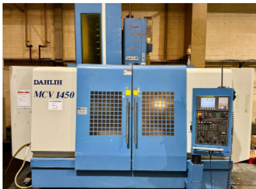
Lot 5: DAHLIH DL-MCV1450 Vertical Machining Centre with Fanuc Series 0i-MC Control (2007)
