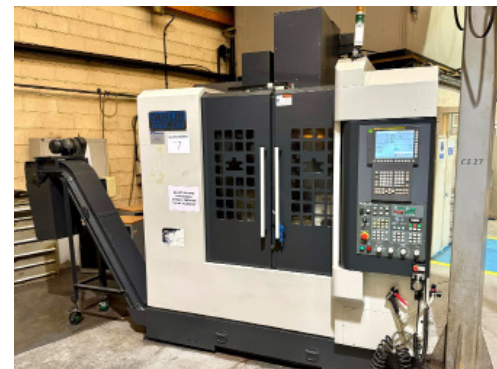
Lot 7: DAHLIH DMX320 5 Axis Vertical Machining Centre with Fanuc Series 0i-MF Control (2018)
