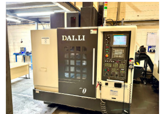
Lot 8: DAHLIH MCV720 Vertical Machining Centre with Fanuc 0i-MD Control (2012)
